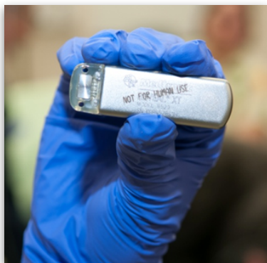
Medtronic Reveal XT 9529, which weighs 15 grams and has a 3 year battery life
